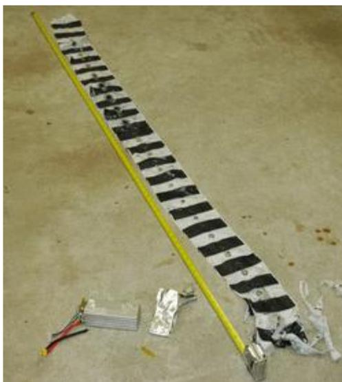
If you ever open up a LiPo foil pouch cell, this is what you will find. A long piece of very thin plastic film (the polymer) with the thin lithium carbon coated aluminum & copper anode & cathode electrodes laminated in an alternating pattern on the front and back side of the polymer separator film. The works will be saturated with the greasy solvent based organic electrolyte.
