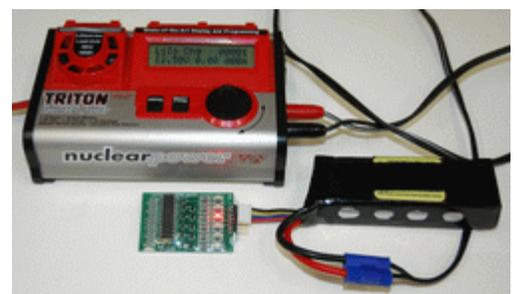
The Blinky will monitor the voltage of each cell in the pack and apply a small load to discharge any cell that is indicating a charge voltage higher than the other cells in the pack keeping all cells within about 0.02 volts (20 mV) of each other.
