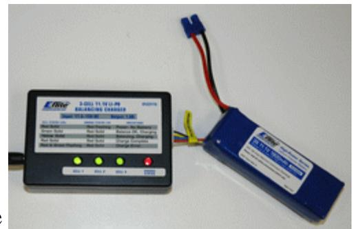
The limitation here is the maximum charge rate. Since the gauge of balance plug wiring is small, this method only works on smaller LiPo's or charge rates not much higher than 2.5 amps maximum. A good clue if you are pushing too many amps through the balance leads would be a warm/hot balance plug/wiring.
